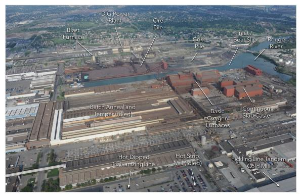
Figure 3 An aerial view of modern-day Dearborn Works, looking Eastward. The facility's hot dipped galvanizing line, hot strip mill, and pickling line tandem cold mill are out-of-frame on the West side of the facility. A portion of the land in the image foreground belongs to Ford. Credit: CLUI
